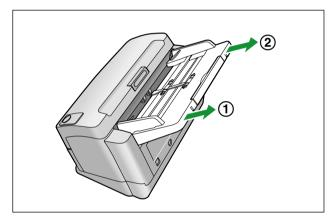
4. Put the mixed batch card guide into the accessory box.
