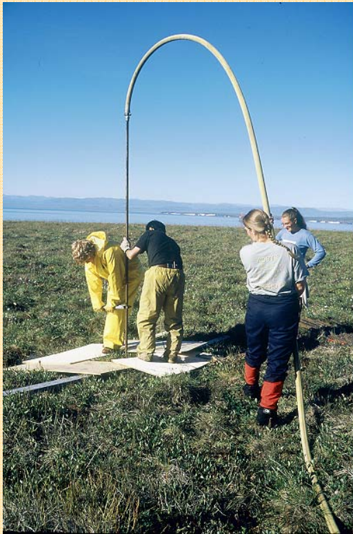
Installation of ground temperature cable, Herschel Island
