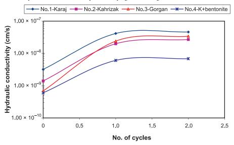
specimens. There were other visible cracks that were not necessarily measurable because of their extremely small size and shape. Thus, the specimens did not have discernible intact portions arguing. The hydraulic conductivity reported is the bulk value and shows an overall increase compared with the hydraulic conductivity of the initial specimen before subjection to drying and wetting cycles.
