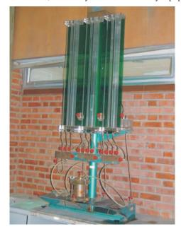
complete cycle of measurement on a specimen consisted of testing for hydraulic conductivity, drying and saturating the specimen, and then repeating the hydraulic conductivity measurement. A hydraulic gradient of 20 was used in the tests (Fig. 2).
