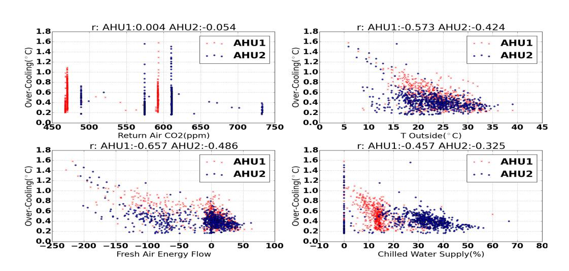
This is a chart showing the correlation between over-cooling and various HVAC related variables. We could visually identify the origin of the overcooling problem: the HVAC system is taking in too much cold outside fresh air when not needed.
