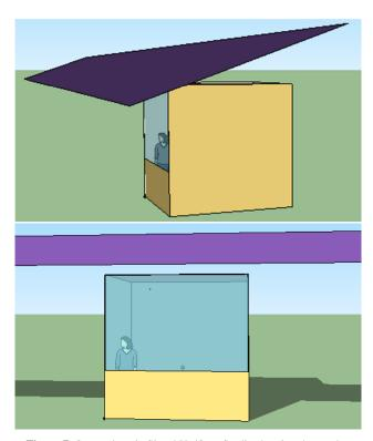
**Figure 7:** Screenshots in SketchUp/OpenStudio showing the south-facing single-occupancy office and fixed shading device.
