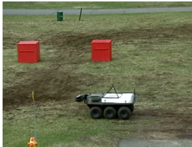
Figure 4.20 Mobile robot carries out the patrol task using Map Data Server component
