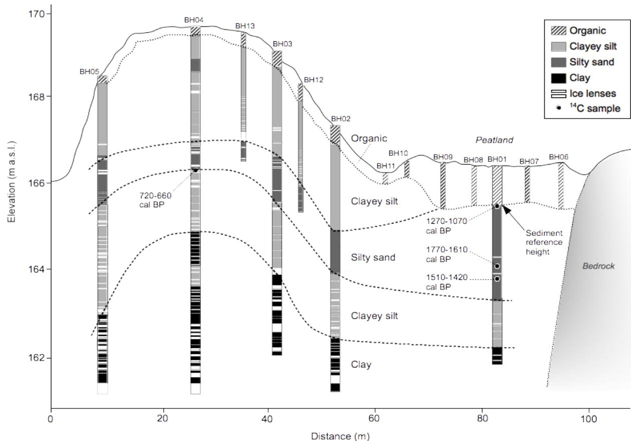
Figure 2. Cross-section of lithalsa at BCSA, displaying all boreholes, ground ice thicknesses, and interpolated stratigraphy.
