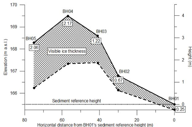
Figure 4. Borehole elevation (with organic cover removed), and distance from BH01, with total thickness of visible ice in each borehole. The reference height is the top of mineral sediment at BH01 in the peatland.
