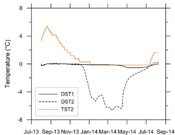
Figure 6. Ground temperatures at 1 m depth at three road sites. For clarity, data from the other road sites are not plotted because they are similar to DST1 and TST2.
