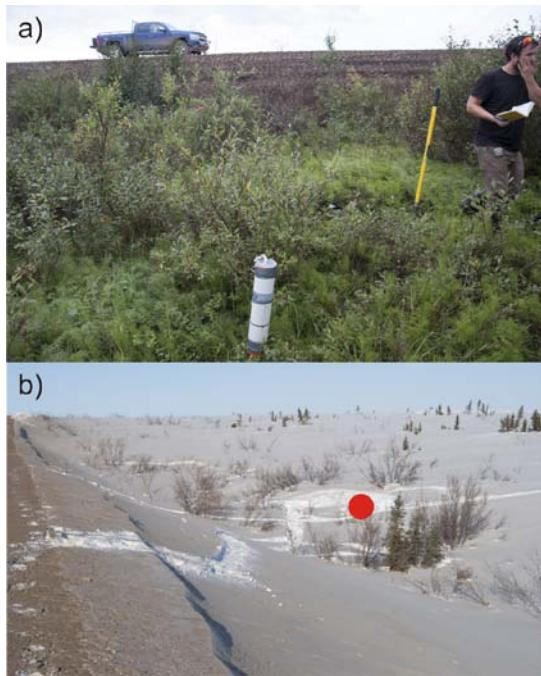
Figure 3. Site TST2 near the highway embankment showing a) the thermistor cable installation and embankment in summer, and b) snow accumulation in winter. Note that many of the tall shrubs are covered by deep snow in winter. The red dot indicates the location of the thermistor cable.
