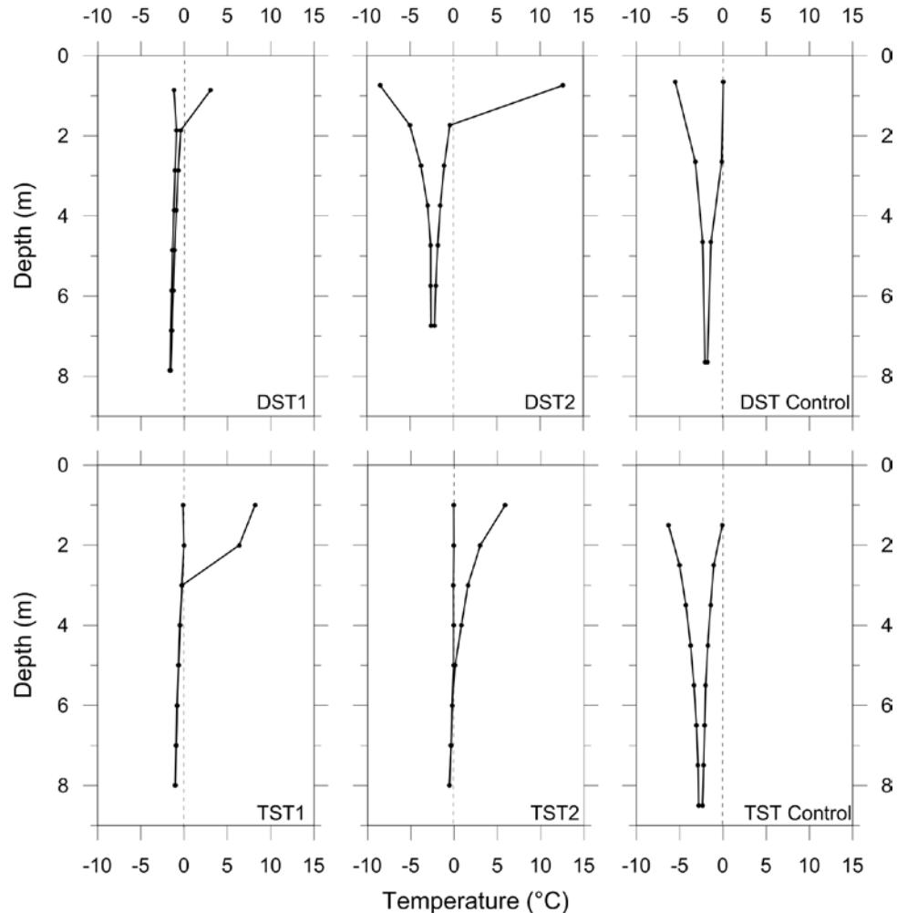
Figure 4. Temperature envelopes for all sites in 2013-14. The dots on the lines indicate the position of thermistors. Note that DST3 is not plotted here.
