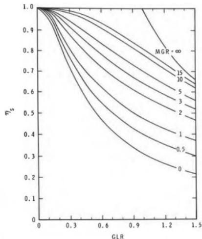
Figure 5. Seasonal solar utilization factor (room temperature swing = 2.75°C)
