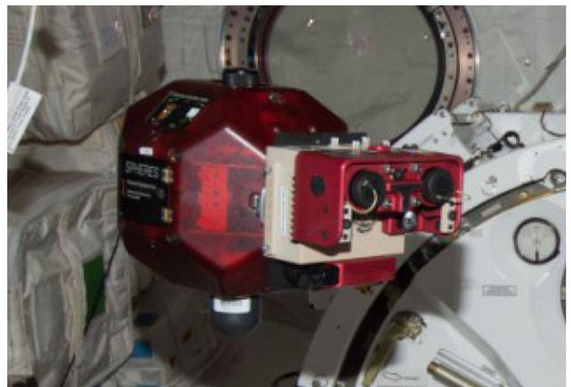
**Fig. 3** SPHERES satellite equipped with the VERTIGO Goggles operating onboard the ISS.
