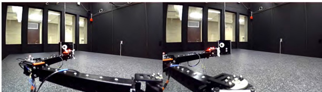
Fig. 4 Example stereo camera imagery with robotic arm extended partially occluding the frame.
