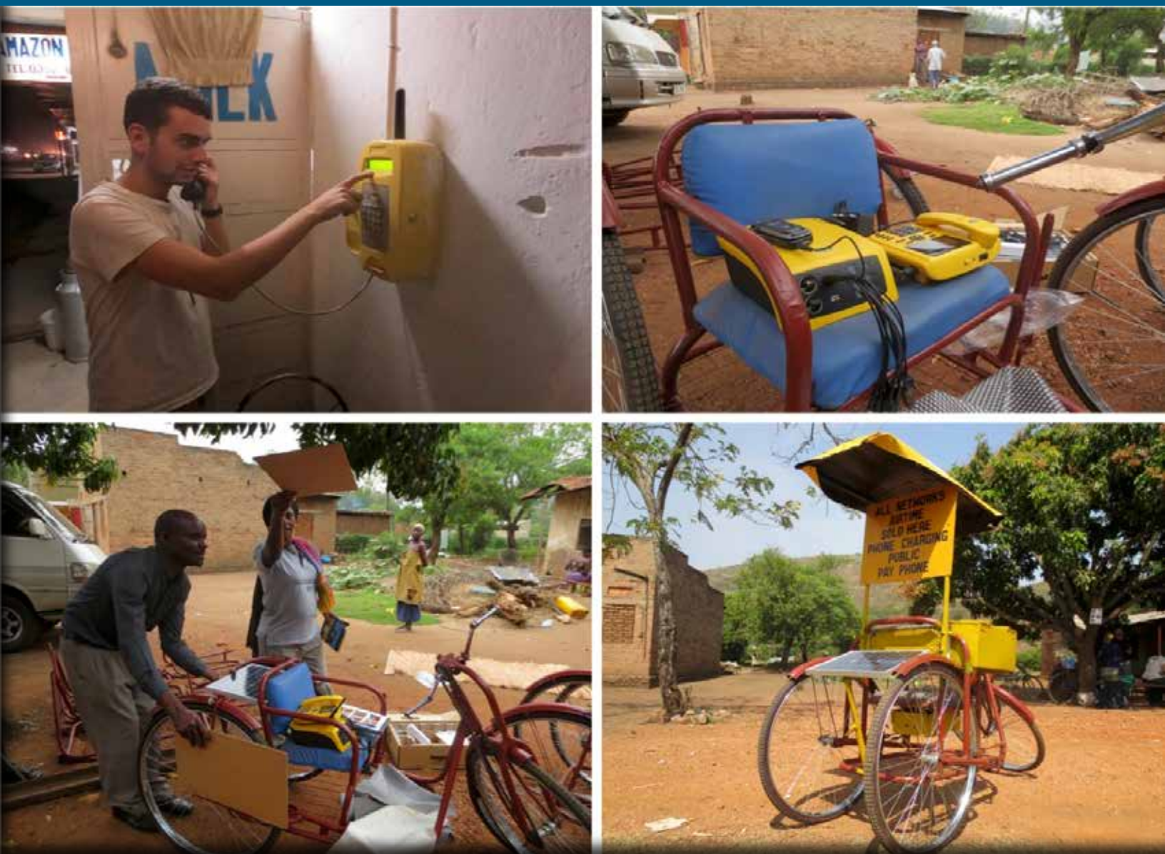
Figure 2: Solar Charging Tricycle (Photos courtesy of Andrew Theobald)
