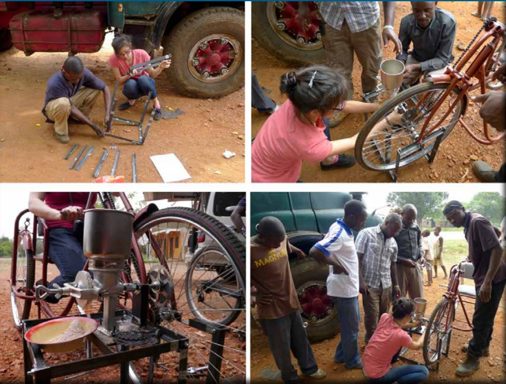
Figure 3. Maize grinder adapted to tricycle hand pedal (Photos courtesy of Carmen Liu)
