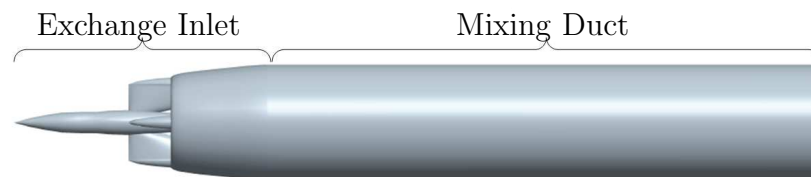
Figure 29: Exchange Inlet and Mixing Duct
