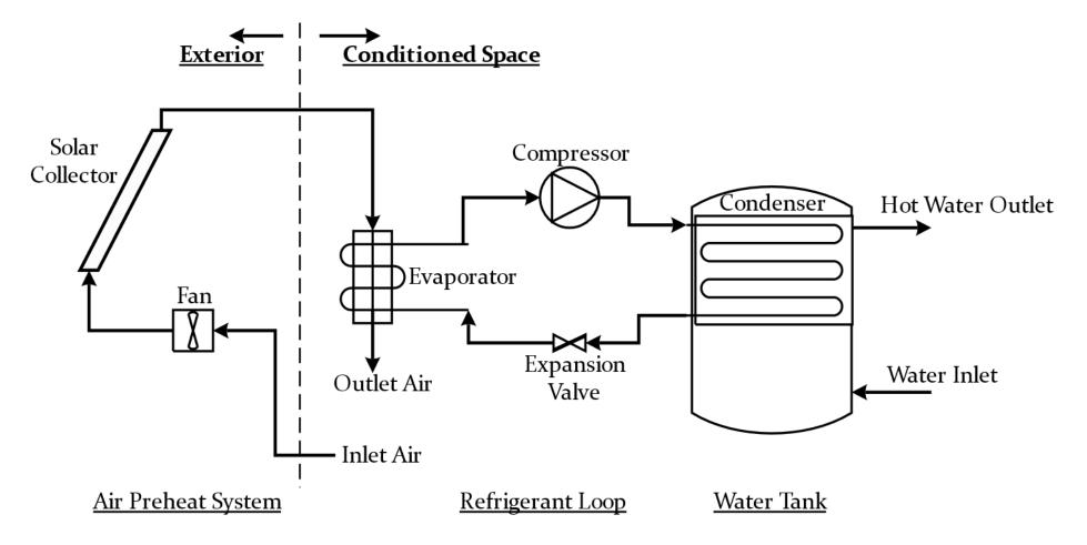
Has impact on space heating and cooling like HPWH-only system
