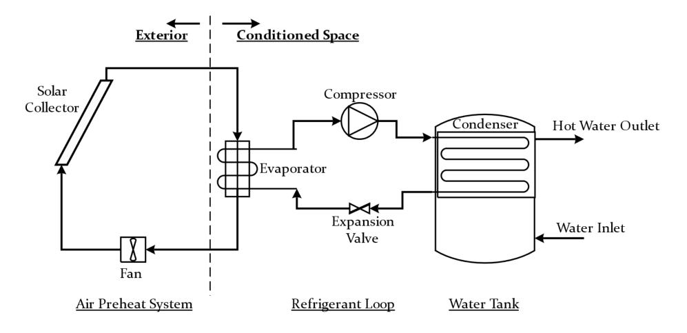
HPWH only operates when inlet temperature (collector outlet) sufficiently high
