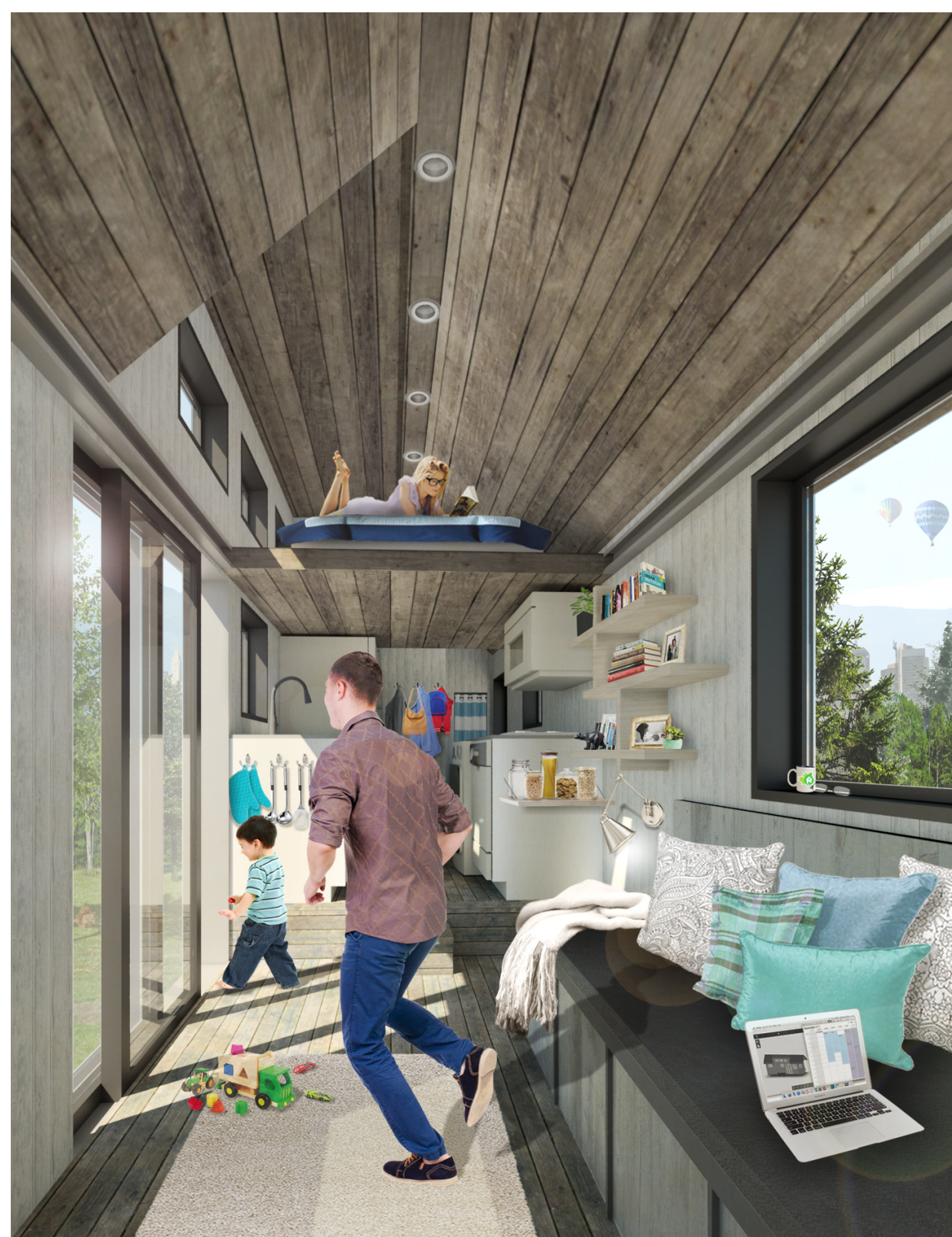
THE OVERHEAD LOFT CAN SLIDE ALONG HORIZONTAL TRACKS IN ORDER TO ADAPT TO DIFFERENT USES OF THE INTERIOR SPACE.
