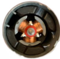
Fig. 8. Internal structure of DC motor
