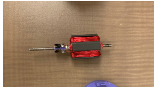
Fig. 13. 3D printed Rotor with Copper Windings
