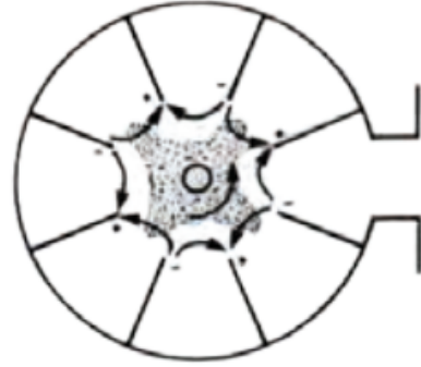
Fig. 3. Spoke Formation of Electrons in the Magnetron [6]
