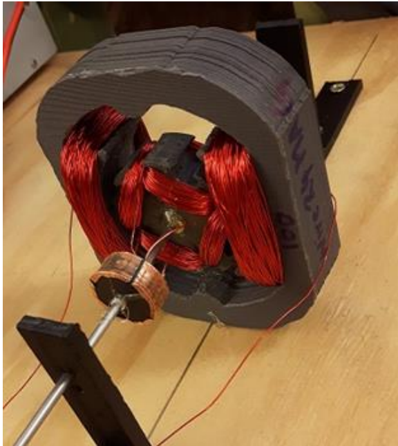
Figure 3: Closed Geometry Self-excited DC Motor (Pole Shoes Made of Magnetic Iron PLA).
