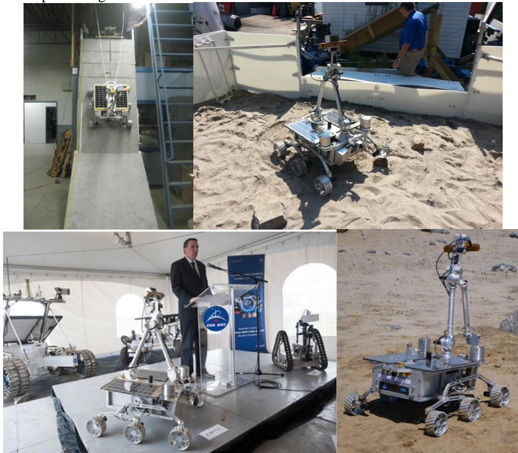
Fig 6. Kapvik micro-rover: Kapvik undergoing cliff abseiling tests; Kapvik undergoing traction tests in a sandbox; Kapvik on display in front of Canada's Minister for Industry Christian Paradis; Kapvik on deployment at Canadian Space Agency's Mars Yard
