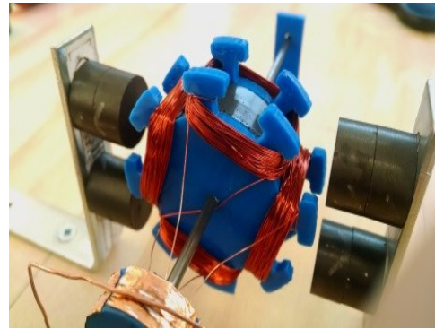
Fig. 7 (a) 3D printed PLA rotor with 50% iron powder by mass; (b) powder metallurgy-manufactured PLA motor with 50% iron powder by volume
