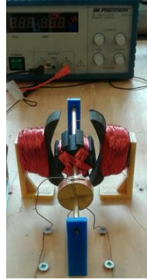
Figure 5b: 3D-printed Stator of Soft Magnetic Steel Source: Ellery 2017
