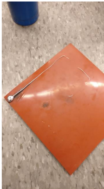
Figure 6: Molten Aluminum Deposited Directly onto Silicone Plastic Source: Ellery 2017
