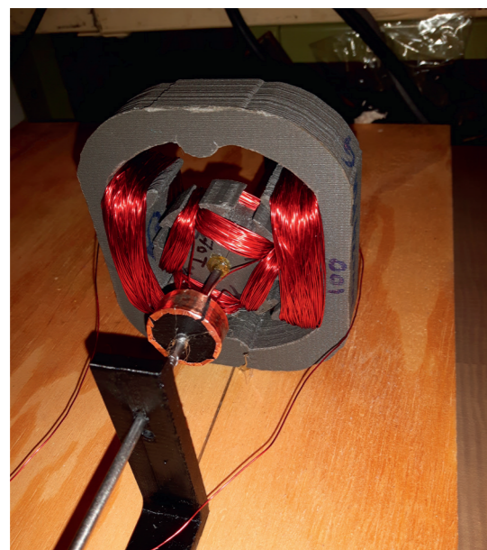
3D printed electric motor (except wire coils)
