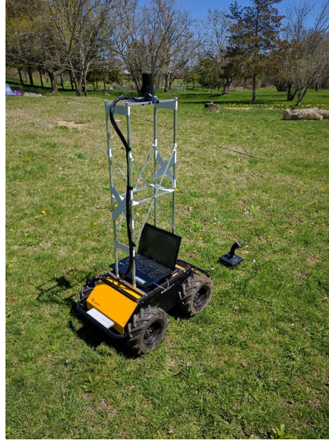
Fig. 1. Photograph of the Husky A200 UGV in survey configuration. A field laptop was employed for troubleshooting and monitoring but was not integral to the operation of the system.
