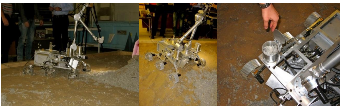
Fig 4. Kapvik using its scoop to acquire regolith deposited into sample canisters
