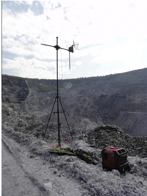
Fig. 4. Wireless network antenna at the Jeffery mine. Its location is indicated in Fig. 1.
