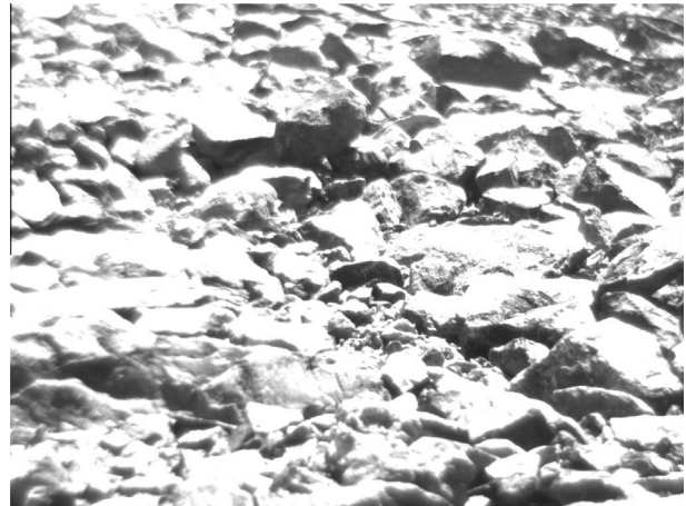
Fig. 18. UV band image of the ground surface from three-band UV–vis imager acquired at the Norbestos site. The field of view is approximately 40 cm across.
