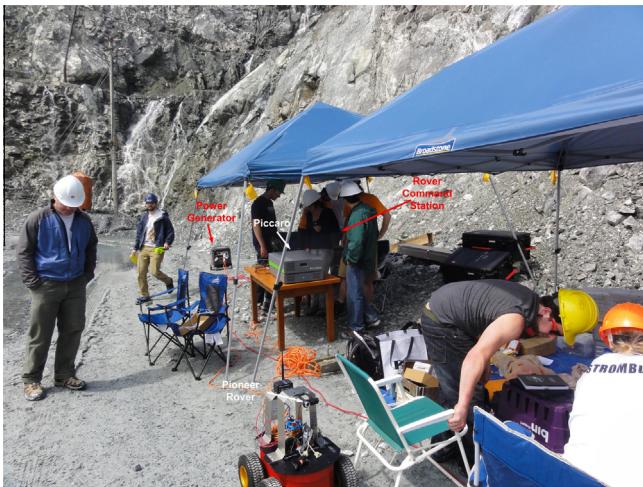
Fig. 6. Base station set up showing Pioneer rover and Picarro sensor at the Jeffrey mine test site.
