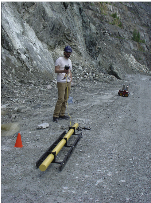
Fig. 3. EMIS mounted on a fiberglass with Pioneer rover in the background (mine test site).
