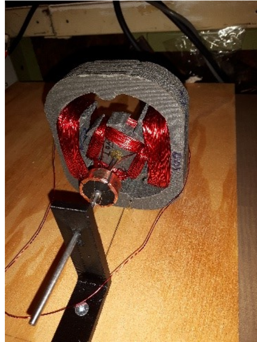
Fig. 1. DC electric motors with 3D printed stator and rotor electromagnets
