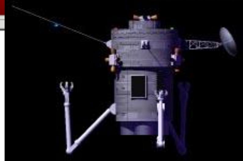
ATLAS dual-arm servicer concept to perform simple repairs on satellites
