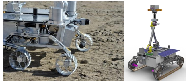
Fig 1. (a) Kapvik instrumented rocker-bogie chassis (actual); (b) Kapvik with elastic loop mobility system (model)
