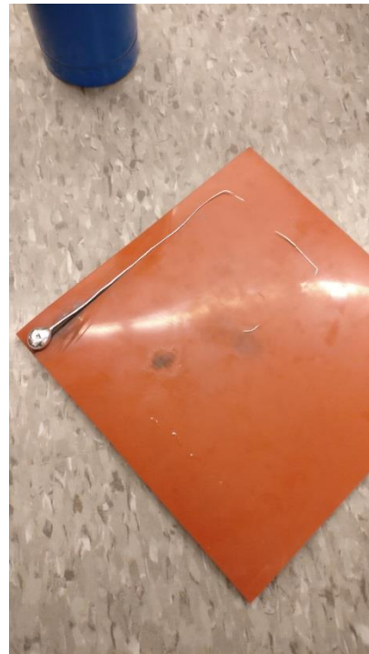
Fig 5. Aluminium track on silicone plastic substrate
