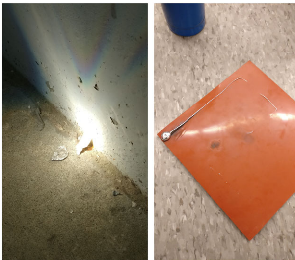
Fig. 1. (a) Fresnel lens melting of aluminium alloy; (b) molten aluminium directly on silicone plastic.
