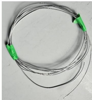
Fig. 13. Shows the Al wire made from the reaction products. It is shown that it was possible to make a spool with this wire.
