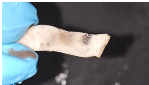
Fig. 10. First Al spheres obtained from the reaction. The pictures show the first Al spheres that were detached from the \text{Al}_2\text{O}_3 pellet. The spheres were very small and were found while rinsing the reaction products with deionized water.
