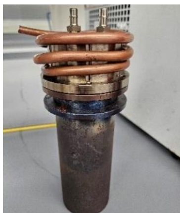
Fig. 4. Coloration contrast between the retort body and lid post-heating. This image shows the difference in coloration between the retort body and the lid after heating. The vessel shows clear signs of heat exposure, while the lid remains undamaged due to the cooling system, preserving its original color.
