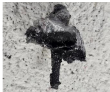
Fig. 6. Damaged graphite electrode. The picture shows a tip which was found in the solidified electrolyte indicating corrosion of the graphite rod and suggesting a reaction between graphite and oxygen in the headspace.
