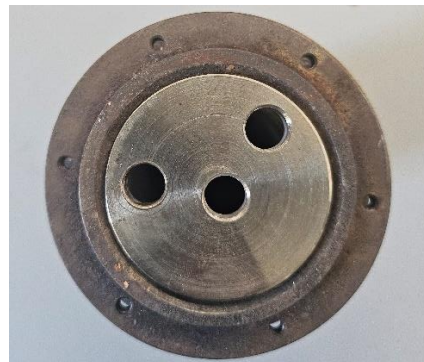
Fig. 1. Top view of the retort and the stainless steel heat shield. The heat shield is shown in the centre in a lighter colour. The heat shield has three holes for the two electrodes and a thermocouple and covers the heating enclosure preventing heat from reaching the lid.
