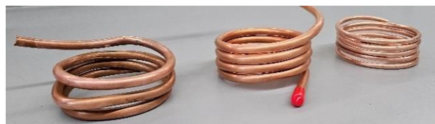
Fig. 2. Copper coils used for the cooling system. Copper tubing of different diameters is shown (3/8in, 1/4in, and 1/6 in from left to right). As the diameter of the tubing decreases, it can coil more times around the lid.
