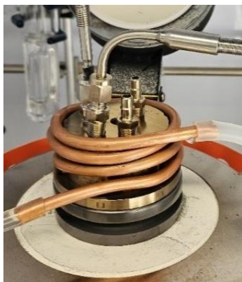
Fig. 3. Cooling system testing. The image shows the cooling system featuring copper tubing during one of the initial tests with the 3/8-inch copper tubing coil around the lid. Two thermocouples are located on the top of the lid. The one located at the back is a long thermocouple that is immersed in the retort, while the thermocouple located at the front is just a superficial thermocouple which is only in contact with the lid.
