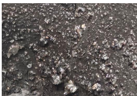
Fig. 17. Powdered products obtained from the electrolysis of an LHS-1 sample. Two main phases were observed: a fine black powder and bigger particles with a metallic finish.
