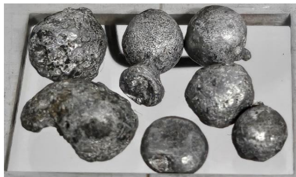
Fig. 11. Al spherules obtained from the electrochemical process. The spherules are placed in a sample holder. These spheres were the result of the best parameter optimization achieved so far. The increase in size is considerable with respect to the spheres of Fig. 10.
