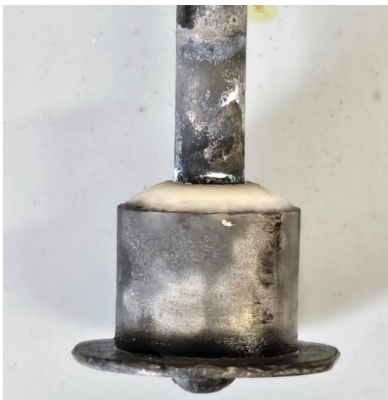
Fig. 8. \text{Al}_2\text{O}_3 pellet coated with Al after the electrochemical process. The image shows early promising results. A metallic coating was formed around the pellet. Only the outside of the pellet had a metallic finish, while the body of the pellet was unchanged.
