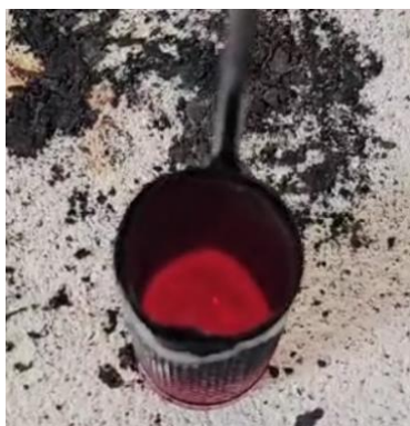
Fig. 14. Beneficiated LHS-1 held by the basket electrode at 950^\circ\text{C} . The figure shows the electrode after being temporarily taken out of the reactor. The beneficiated LHS-1 can be seen as a red hot material retained by the electrode basket.
