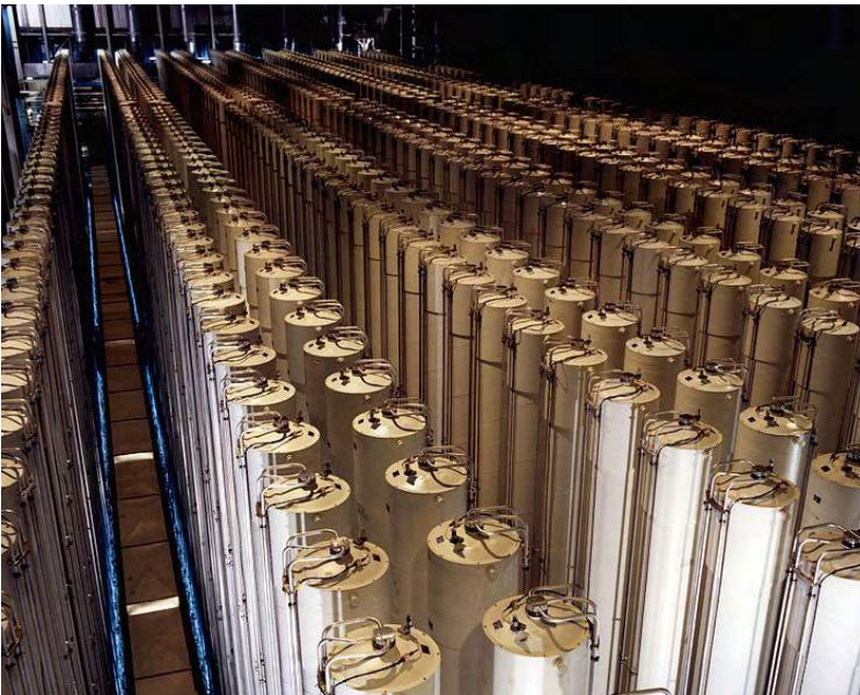
Gas centrifuges like the ones destroyed by Stuxnet. Courtesy of CartoonPeril2011 on Flickr.
