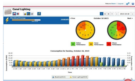
Figure 1. The existing building dashboard interface implemented at Carleton University
