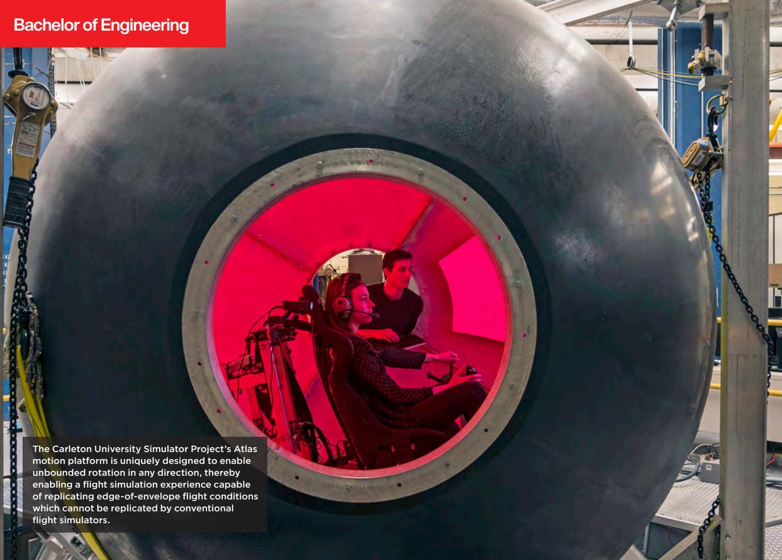
The Carleton University Simulator Project's Atlas motion platform is uniquely designed to enable unbounded rotation in any direction, thereby enabling a flight simulation experience capable of replicating edge-of-envelope flight conditions which cannot be replicated by conventional flight simulators.
