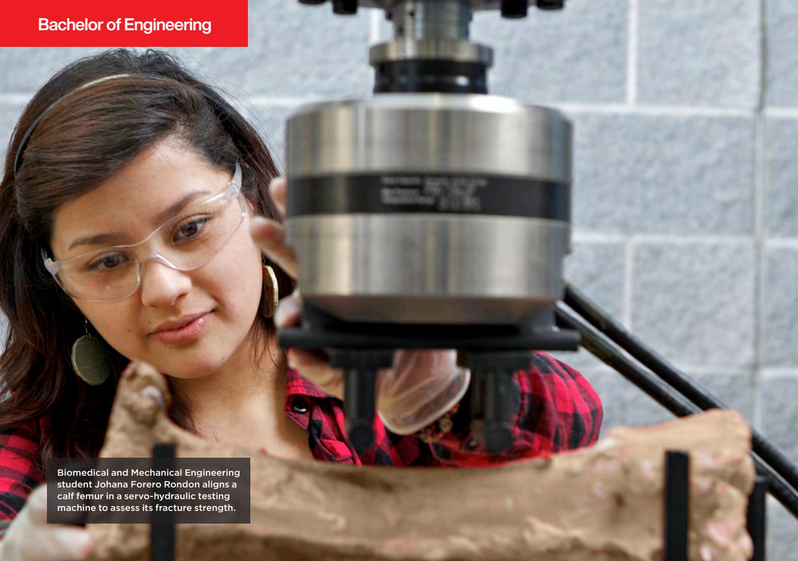
Biomedical and Mechanical Engineering student Johana Forero Rondon aligns a calf femur in a servo-hydraulic testing machine to assess its fracture strength.
