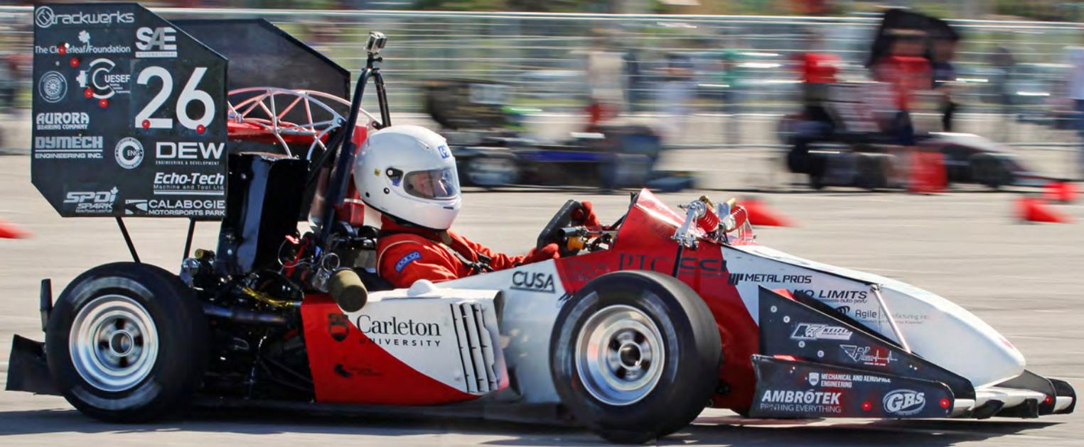
Each year, Carleton's Ravens Racing competes against hundreds of teams from around the world in the international Formula SAE series. The team's newest Formula SAE vehicle, designed and constructed by students from a variety of engineering disciplines and powered by a 50 horsepower engine, can accelerate from 0 to 100 in 4.5 seconds and reach speeds of up to 120 km/h. During the 2019 season, the team found record success, earning multiple podium and top ten finishes.
