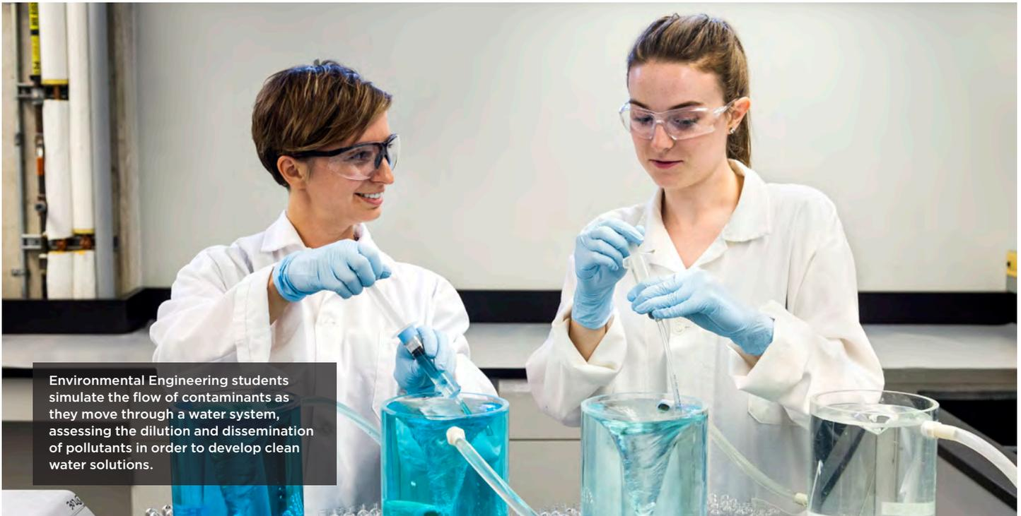
Environmental Engineering students simulate the flow of contaminants as they move through a water system, assessing the dilution and dissemination of pollutants in order to develop clean water solutions.
