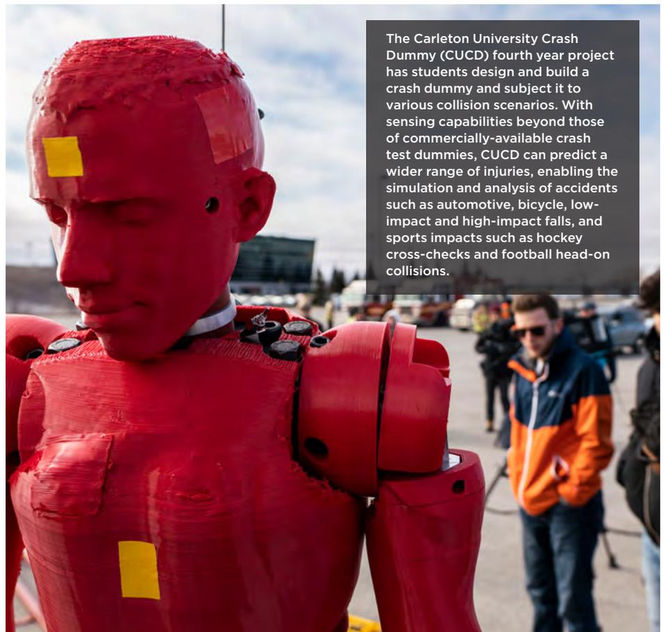
The Carleton University Crash Dummy (CUCD) fourth year project has students design and build a crash dummy and subject it to various collision scenarios. With sensing capabilities beyond those of commercially-available crash test dummies, CUCD can predict a wider range of injuries, enabling the simulation and analysis of accidents such as automotive, bicycle, low-impact and high-impact falls, and sports impacts such as hockey cross-checks and football head-on collisions.
