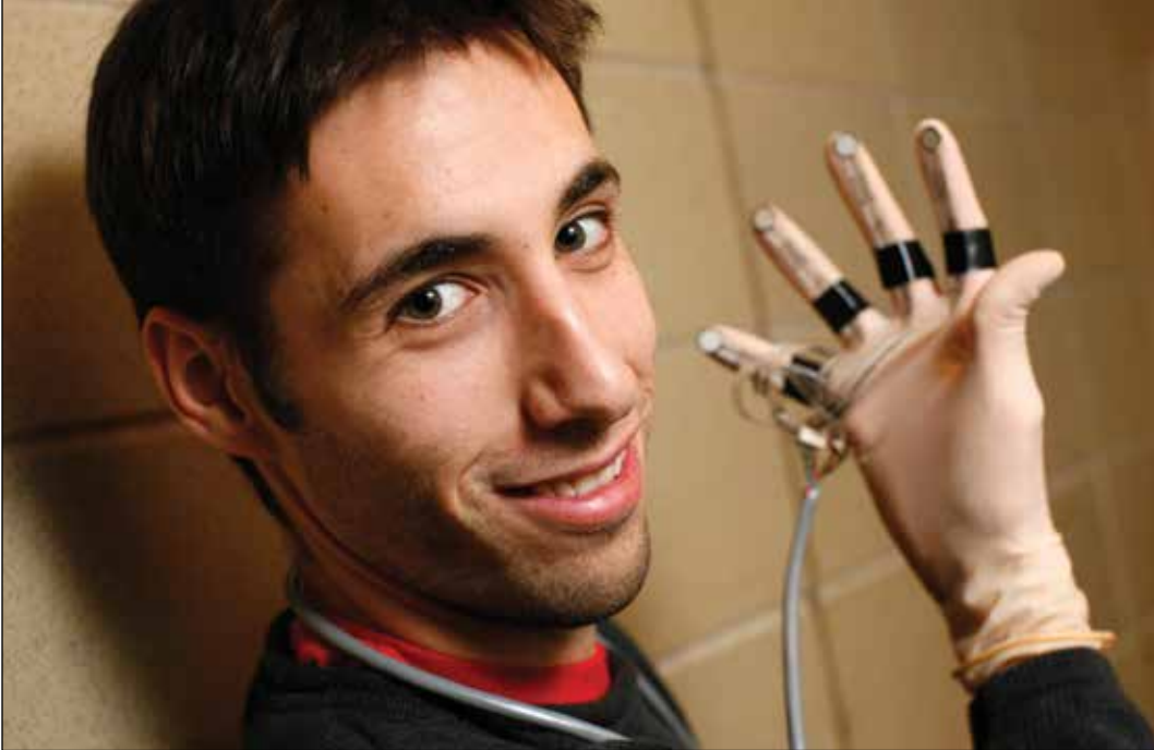
Carleton graduate student Andrew Geddes developed a device to measure the position and force of a doctor's fingertips during abdominal examinations.
