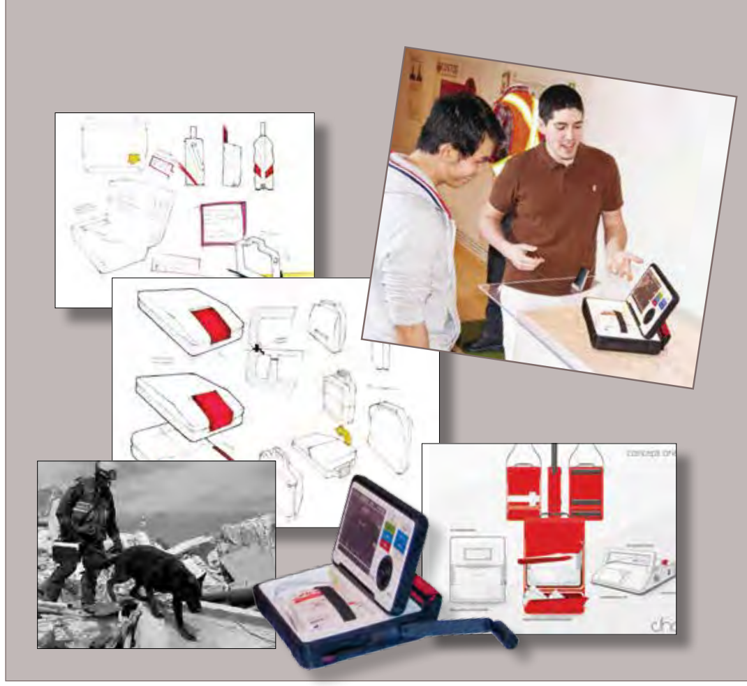
Fourth-year student Ian Murchison developed a portable defibrillator with its own power source which could be used by medical professionals working in the field (for example, on earthquake rescue missions).
