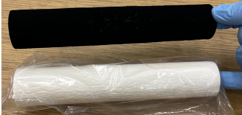
Figure 3.5: Two filters that are used in the sampling line before the vacuum pump. The top filter (black) is after a days-worth of flame testing, and the bottom filter (white) is an unopened replacement. The blackness seen on the top filter is soot cake build-up filtered out of the exhaust flow before passing through the MFC and vacuum pump. As the soot builds up, flow is restricted through the vacuum.
