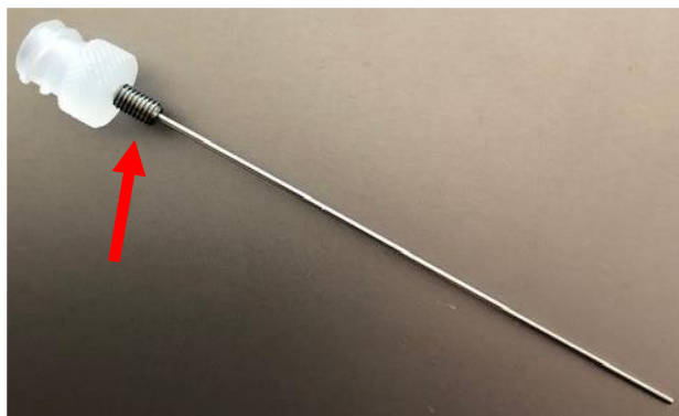
Figure 2.4: LS-FSR fuel supply capillary with a threaded modification to improve precise positioning and consistency in co-flow of the liquid fuel and surround dispersion oxygen.
