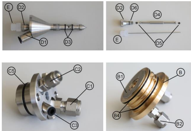
Figure 2.3: Central insert and liquid fuel supply capillary (top) and the central body with sheath gas homogenizer (bottom). Table 2.1 identifies labeled parts for the central inserts, capillary, and homogenizer [53].
