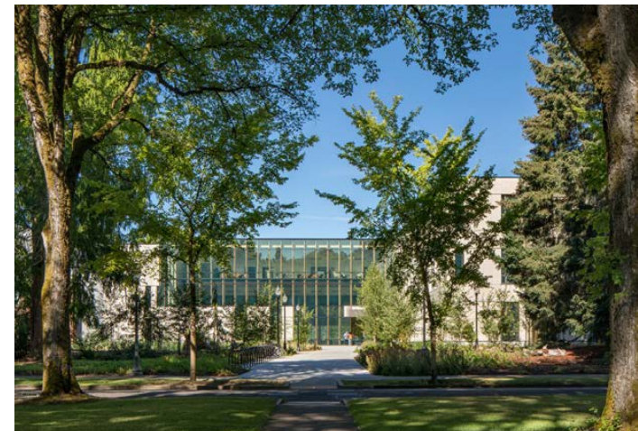
Buildings framing green spaces should have generous ground floor setbacks filled with native planting and vegetation to create a comfortable micro-climate for pedestrians. (Oregon Forest Science Complex, Michael Green Architecture © Josh Partee)
