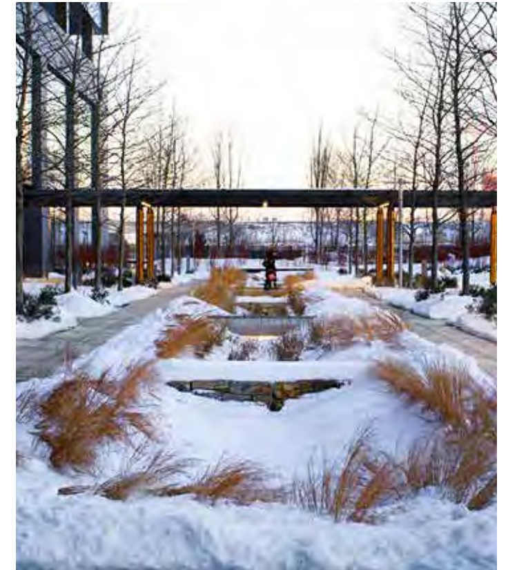
In the winter, rain gardens and bioswales can create seasonal interest and become designated areas that require less maintenance. (Somerville, Massachusetts, OJB © Andrew Cridlin)
