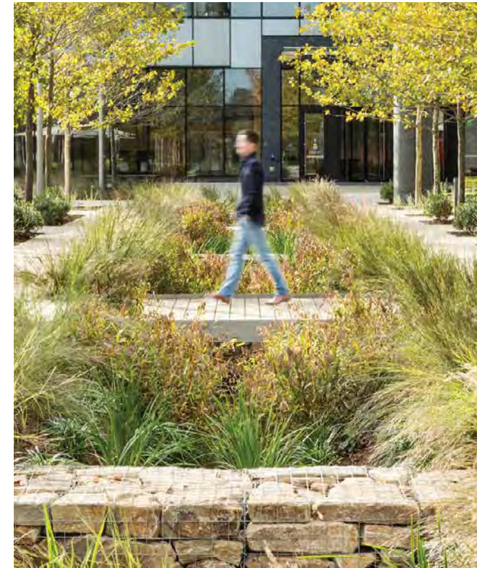
Rain gardens collect stormwater runoff and are often planted with native species that do not require permanent irrigation. (Somerville, Massachusetts, OJB © Kyle Cadwell)
