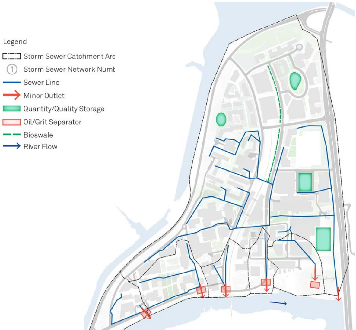
Diagram showing storm sewer and quality/quantity control
