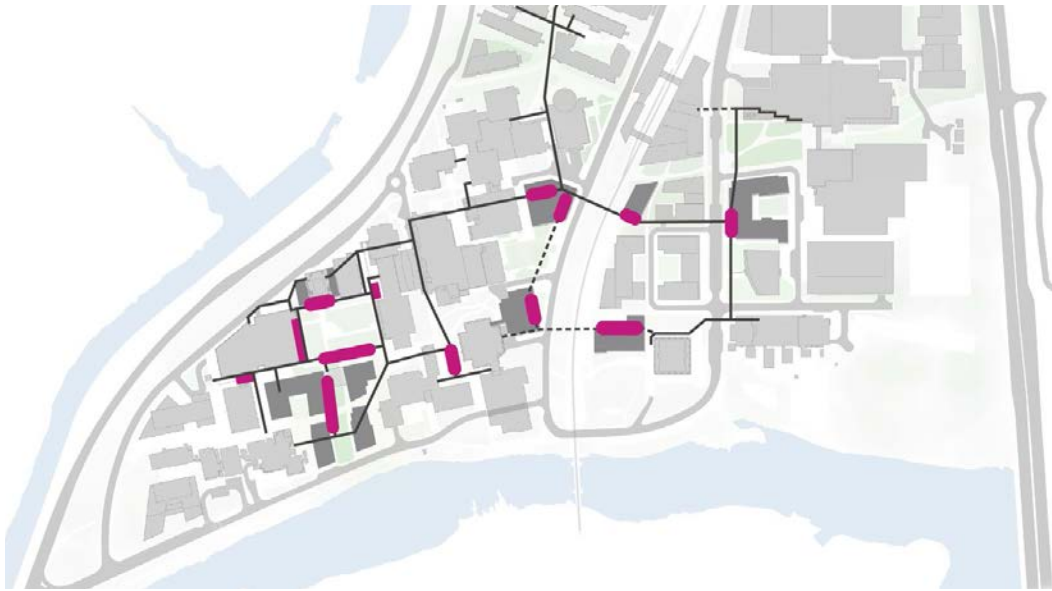
Map identifies areas where tunnel improvements should be considered in the academic core. Improvements include incorporating daylighting (purple) and better connectivity (dashed black)
