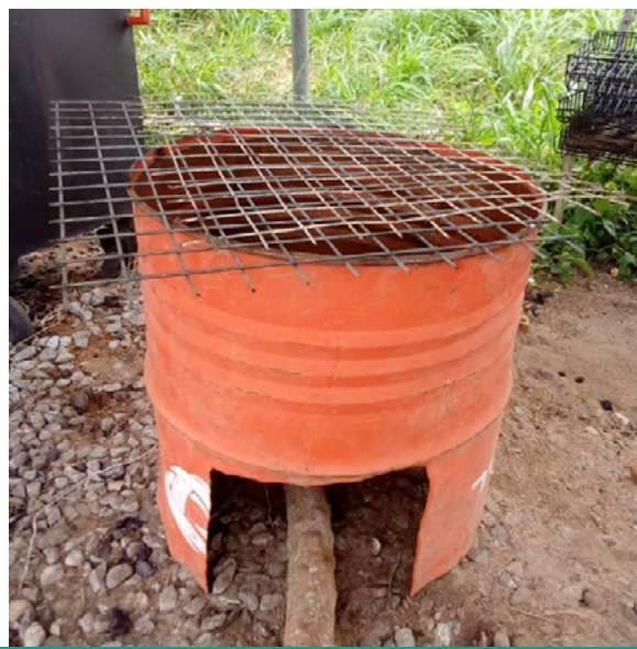
A half-drum smoking kiln built during the research design process.
