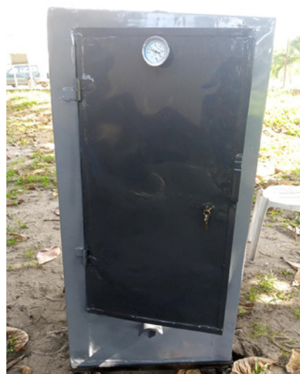
External view of a fabricated charcoal-fired smoking kiln of 80 kg production capacity built during the research design process.
