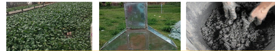
Left to right: Water-hyacinth ( Eicchornea crassipes ) at the jetty on Ojo Creek, used for the production of briquettes; Picture of one of the first hybrid fish dryer prototypes combining both solar and biomass fuel in one component; Mixing of biofuel materials with cassava starch for briquette production.
