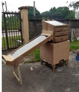
Early prototype of a hybrid solar-biomass fish dryer.
