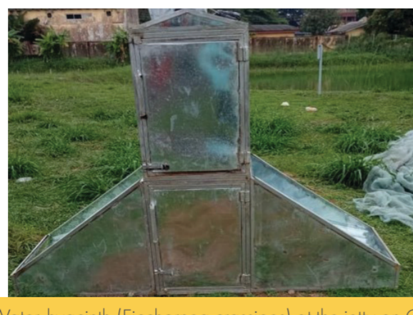
Left to right: Water-hyacinth ( Eichhornia crassipes ) at the jetty on Ojo Creek, used for the production of briquettes; Picture of one of the first hybrid fish dryer prototypes combining both solar and biomass fuel in one component; Mixing of biofuel materials with cassava starch for briquette production.
