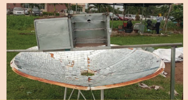
Top to bottom: Modern smoking kiln with charcoal pot in smoking chamber and chimney at the top; Parabolic Dish Solar Collector with Fish Drying Chamber open to show Copper Plate at the base.
