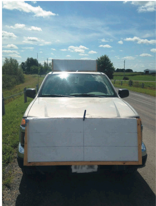
Figure 1. Vehicle-mounted sticky traps attached to the front grill ( 0.5 \times 1.2 m area) and roof ( 0.3 \times 1.2 m) of a pickup truck. A sticky trap had a plywood frame which was secured to the truck using ratcheting straps. We inserted a thin board covered in heavy plastic wrap into that frame and applied Pestick (Phytotronics, Inc., Earth City, Missouri, USA) to the exposed area of plastic wrap. The surface area of each trap was subdivided into six equal-area portions.
