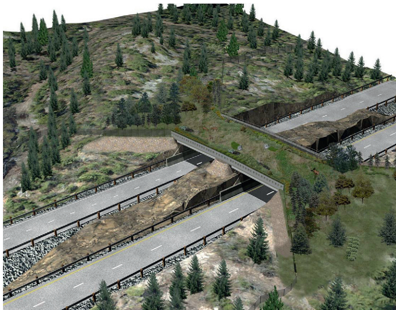
Figure 2. Schematic representation of a vegetated overpass on Highway 69 in Ontario, Canada. Early collaboration between planners and researchers led to the design of a 30 m-wide overpass to accommodate the large population of elk, Cervus elaphus , and other large mammals present in the area. This overpass and the road were completed in 2012. Reproduced, with permission, from the Ontario Ministry of Transport.
