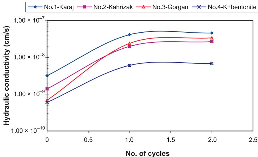
specimens. There were other visible cracks that were not necessarily measurable because of their extremely small size and shape. Thus, the specimens did not have discernible intact portions arguing. The hydraulic conductivity reported is the bulk value and shows an overall increase compared with the hydraulic conductivity of the initial specimen before subsection to drying and wetting cycles.
