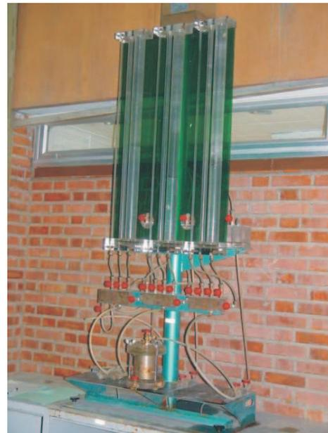
complete cycle of measurement on a specimen consisted of testing for hydraulic conductivity, drying and saturating the specimen, and then repeating the hydraulic conductivity measurement. A hydraulic gradient of 20 was used in the tests (Fig. 2).
