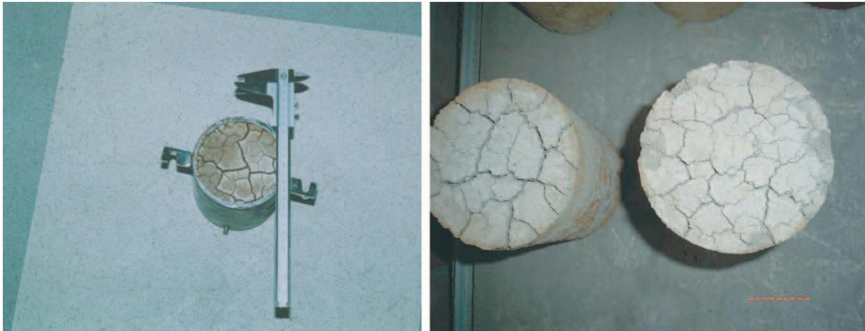
**Table 2.** Volume change – cracking records for the soil specimens (dimensions in mm).
