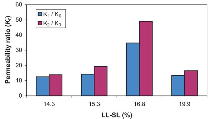
This phenomenon is generally referred to as self-healing. It is believed that the different changes in hydraulic conductivities are associated with self-healing processes that affect the various soil types by different degrees (Eigenbrod 2003). Therefore, one of the goals of the present study was to investigate the behavior of self-healing in different clayey soils.
