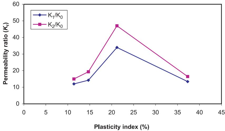
mately 35 times its initial hydraulic conductivity. The permeability ratio shows a decrease to about 13 ( $K_1/K_0 = 13.4$ ) with an increase in plasticity index of 37.3% for sample 4, which could be due to the effect of self-healing on the permeability behaviour in high plasticity soils. This behavior is similar to the results of other researchers (e.g., Eigenbrod 2003) for fine-grained soils.
