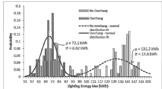
**Figure 10:** Probabilities distributions and normal distribution fits for the lighting energy use for an office with and without a fixed shading device.
