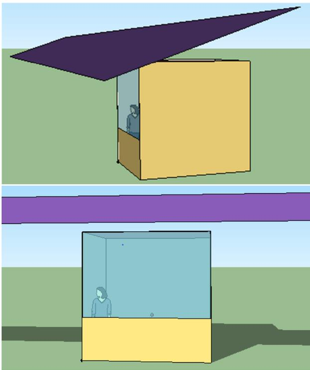
**Figure 7:** Screenshots in SketchUp/OpenStudio showing the south-facing single-occupancy office and fixed shading device.
