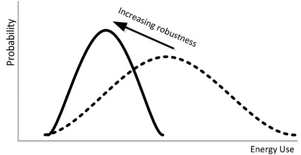
**Figure 3:** Illustration of the robustness concept: lower mean and standard deviation of building performance
