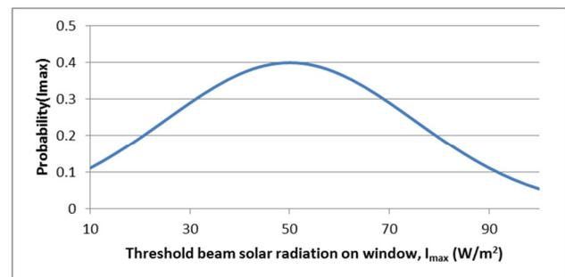
**Figure 9:** Probability distribution for the threshold of solar radiation on the window, above which the occupant closes the shade.
