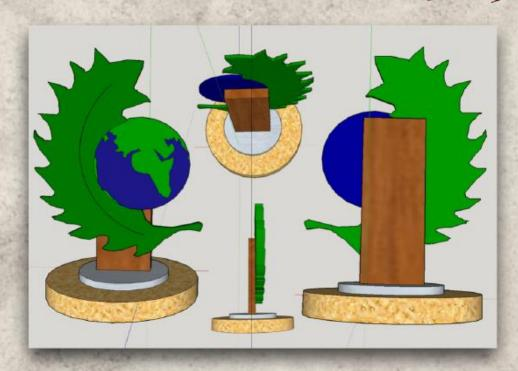
My final product has the earth and leaf form on both sides. (which were both cut out on the laser cutter) The wooden base was cut manually and the title of the trophy was etched around it. I also casted the pewter disc on the base.
