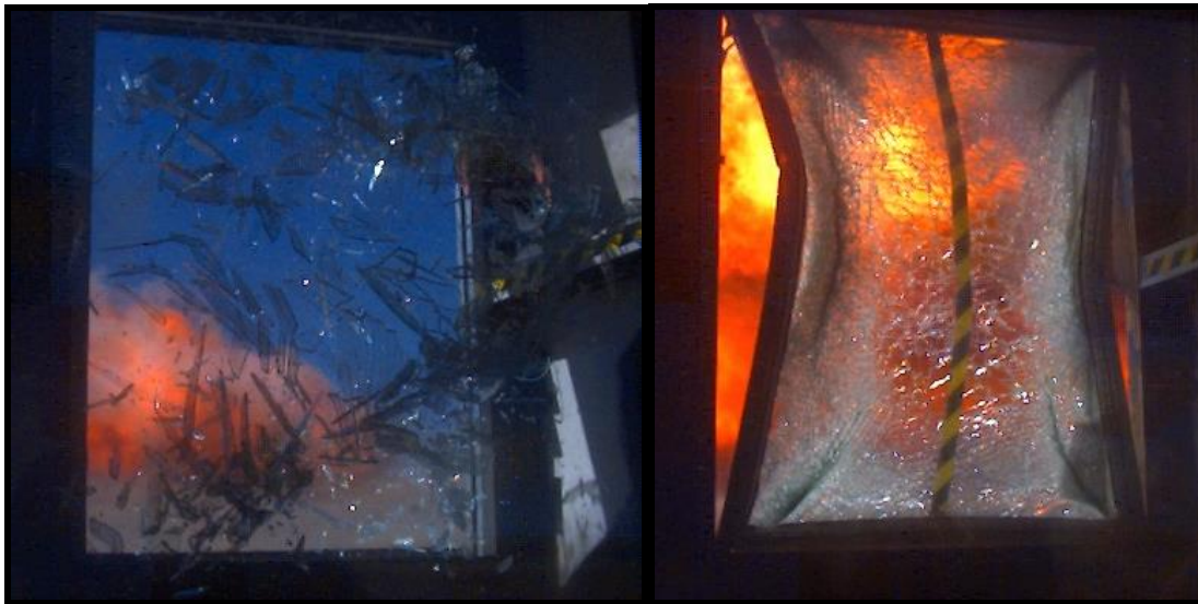
Figure 3: Response of unprotected annealed glass on the left versus filmed glass on the right as viewed from inside a building
