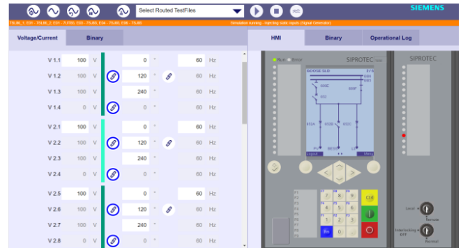
Fig. 5. VELP uses the SIPROTEC Digital Twin platform
