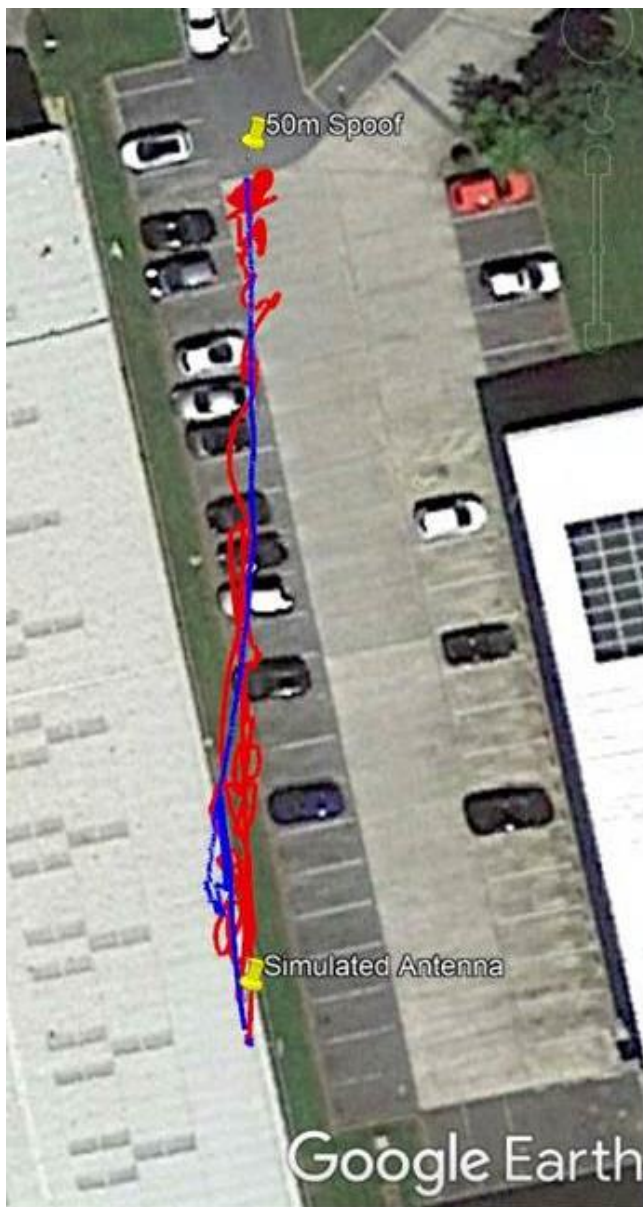
Figure 8: Reported ground tracks of R_1 (red) and R_2 (blue) during the 50m test case (Simulation only).
